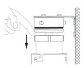
4. If the filter cartridge does not come away with the sump release it with an index finger by pushing down on the plastic rim.
