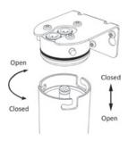
3. Firmly grip the sump with both hands. Turn to the left and pull down. The sump and the filter cartridge should come away together. The filter canister will be full of water so it is advisable to position a bowl to catch any spills.
