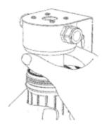
4. Unscrew the filter cartridge until it comes free. Carefully remove the sump with the cartridge inside. Remove the cartridge and discard the water in the sump. Dispose of the spent cartridge.
