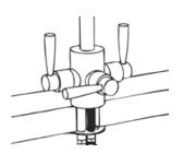
2. Turn on the dispenser to release the pressure in the system. Leave the tap in the 'on' position.\*
