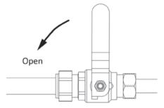
7. Turn the water supply 'on' and check the system carefully for leaks. Leave the filter tap in the 'on' position and allow the water to run for approximately 10 minutes to flush the system. The optimum flow rate is 2 litres per minute. If the flow is too fast it can be regulated by adjusting the stop valve.
