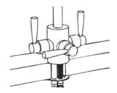
Turn on the dispenser to release the pressure in the system. Leave the tap in the 'on' position.\*
