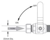
7. Turn the water supply 'on' and check the system carefully for leaks. Leave the filter tap in the 'on' position and allow the water to run for approximately 10 minutes to flush the system. **IMPORTANT NOTE:** The optimum flow rate is 2 litres per minute. The performance of the filter will be negatively affected if the flow rate is too fast. If necessary the flow rate can be regulated by adjusting the stop valve.
