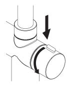
2. Turn the tap's boiling water handle to the "ON" position for a few seconds to release the pressure in the system.
