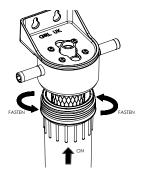
6. Tighten the sump firmly sufficient to make a water tight seal.
