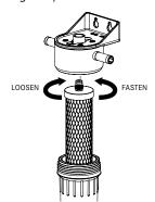
5. Reverse the removal procedure: install the new cartridge, taking care not to Over-tighten it, and refit the sump.
