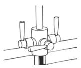
Turn on the dispenser to release the pressure in the system. Leave the tap in the 'on' position.\*
