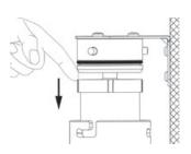
If the filter cartridge does not come away with the sump release it with an index finger by pushing down on the plastic rim.
