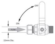
7. Turn the water supply 'on' and check the system carefully for leaks. Leave the filter tap in the 'on' position and allow the water to run for approximately 10 minutes to flush the system. The optimum flow rate is 2 litres per minute. If the flow is too fast it can be regulated by adjusting the stop valve.
