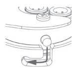
Refit the sump to the housing head by engaging the pins in the slots and turning the sump to the right until it is fully engaged.
