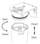
3. The filter cartridge housing will be full of water, so ensure you have a bowl to hand to catch any spills. Turn the lower section (the sump) of the housing to the left and pull down. The sump and the filter cartridge should come away together.
