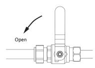
Turn the water supply 'on' and check the system carefully for leaks. Turn on the electricity supply to the boiler.
