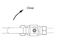
1. Locate the shut-off valve and turn off the mains water supply to the filter housing.
