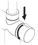
Turn the tap's boiling water handle to the "ON" position for a few seconds to release the pressure in the system.
