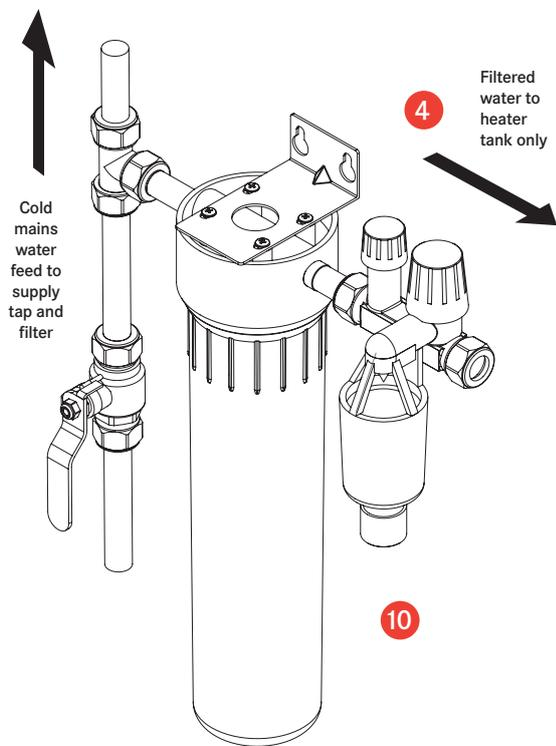
3 Turn the stop valve (the small knob) on the Inlet Pressure Relief Valve to 'OFF' the turn on the mains water supply and check the assembly for leaks, and rectify as necessary. Once this check has been carried out, turn off the mains water supply again. The expansion discharge of the Inlet Pressure Relief Valve and the tundish must always point downwards and remain unobstructed.
