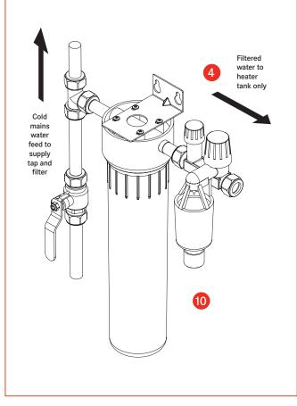
3 Turn the stop valve (the small knob) on the Inlet Pressure Relief Valve to 'OFF' to turn on the mains water supply and check the assembly for leaks, and rectify as necessary. Once this check has been carried out, turn off the mains water supply again. The expansion discharge of the Inlet Pressure Relief Valve and the tundish must always point downwards and remain unobstructed.
